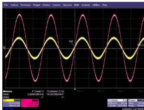
Figure 8.3: OPA227 A_v=50\text{dB} @ 2.2 kHz
