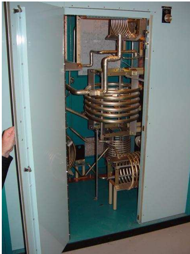
Figure 3.18: High power inductors formed from hollow tubes.
